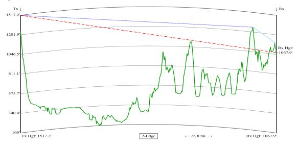
The red line is the line-of-sight that is blocked by the Earth. The blue lines are the shortest path, but the signal doesn't really bend. Each mountain is a 2D slice through a 3D topographic feature. The TV signal can cover a mountain ridge for miles (think into and out of the page,) and every point along the ridge re-radiates signal omni-directionally into the valley
